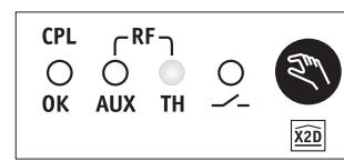
The **AUX** light goes off when the association signal from the door/window sensor has been received
