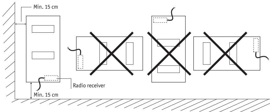
**IMPORTANT** This towel radiator should never be installed with the power supply unit positioned topside. Ensure that the bottom of the towel radiator is positioned at least 15 cm from the floor.
