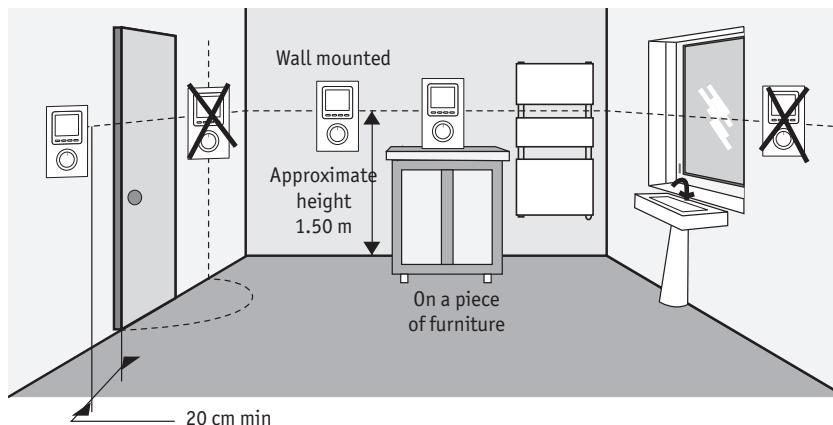
To ensure optimum room temperature regulation, the thermostat must be installed in the same room as the appliance(s) it is controlling.
