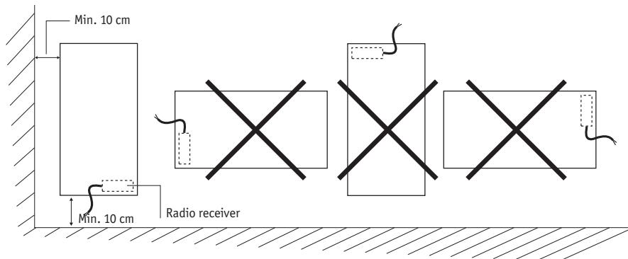
**IMPORTANT** This radiator should never be installed with the power supply unit positioned topside. Ensure that the bottom of the radiator is positioned at least 10 cm from the floor.
