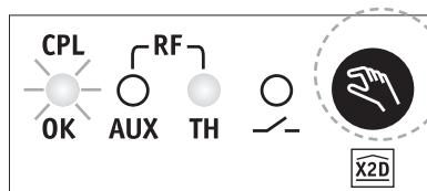
The TH light is glowing steadily (the radiator is associated with the thermostat) and the PLC light is blinking, showing that it is awaiting association with the PLC unit
