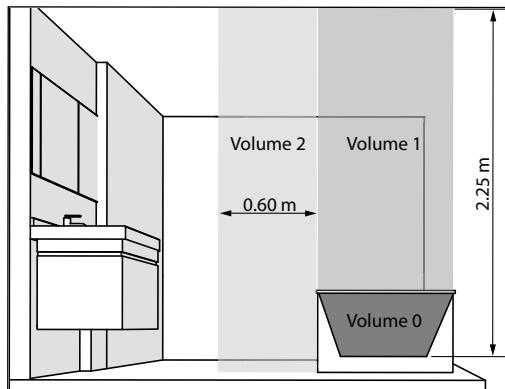
The electricity supply must be protected by a residual current device with a maximum of 30mA, especially when installed in a room containing a bathtub or shower.
